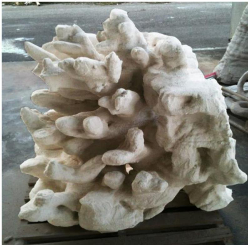
Fig. 1. Three-Dimensional reef unit from a patented sandstone material (SOI, 2012)
